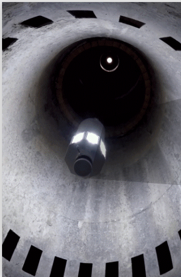
The robotic system ascends and descends in a vertical direction, scanning the interior of the structure
