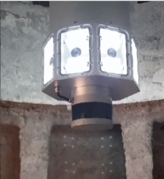
The robotic system ascends and descends in a vertical direction, scanning the interior of the structure
